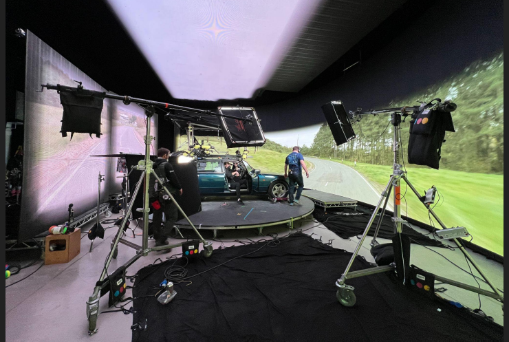
Shot showing the technical setup, the car is located on a turntable surrounded by a 360 degree driving plate.
